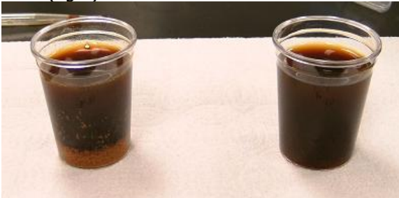
Figure 3. Tea concentrate #3 diluted to approx 7°B. Teas filtered at 17-24°C (left) and at 5-12°C (right).
